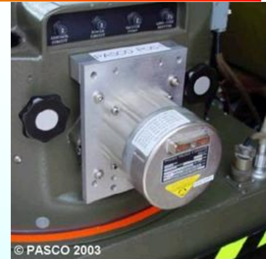
System installation POS/AV test LN200 IMU mounted at RC30 camera
