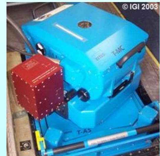
System installation AEROcontrol test IMU-IId mounted at RMK-Top camera
