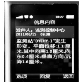
图 9 监测预警信息手机短信自动发布 Fig. 9 Automatic release of mobile phone short message about monitoring and early warning information
