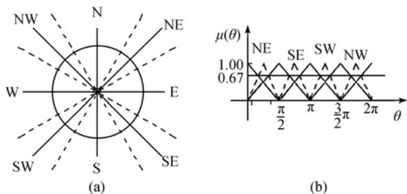
Fig. 2 8-directions fuzzy division in space (a) 8 tiles; (b) Membership functions of each tile
