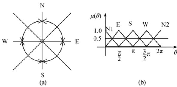
Fig. 1 4-directions fuzzy division in space (a) 4 tiles; (b) Membership functions of each tile
