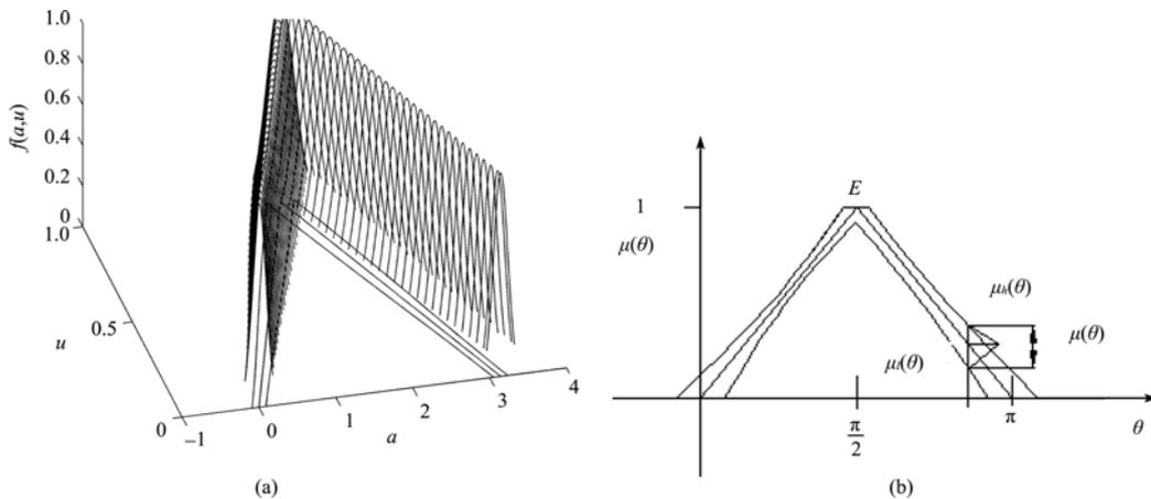
Fig. 4 Type-2 fuzzy set and interval type-2 fuzzy set for east
