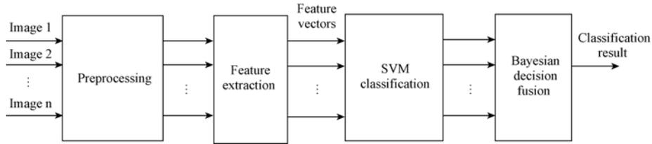
Fig. 1 Process diagram of SAR image target recognition
