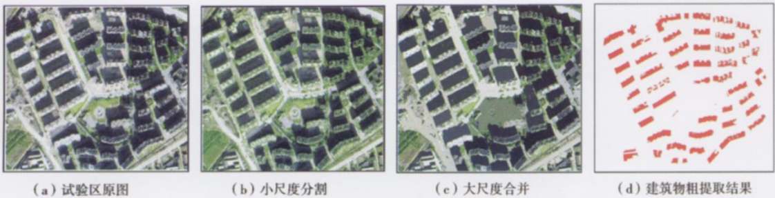
图 3 建筑物矢量图的粗提取 Fig. 3 The process of extracting the building vector coarsely
