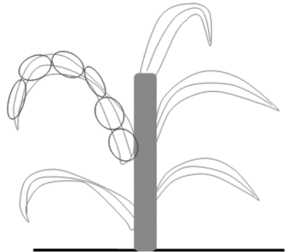
Fig. 2 Corn leaf is treated as assemblage of disc with random orientation
