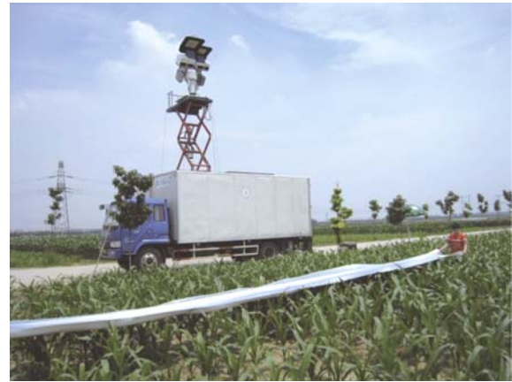
Fig. 4 Corn field experiment by microwave radiometer in July 7 at Qing Yuan, Hebei Province, China
